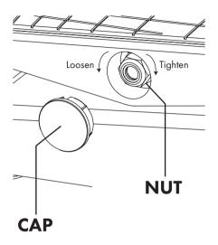
To loosen or tighten rocker movement of pedal, pry cap from right side of pedal with a small flat-head screwdriver; use 10mm socket wrench to adjust nut to pedal motion preference. To avoid damage to pedal assembly, do not over-tighten.
